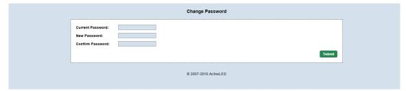
The Change Password submenu allows you to set a password or change a current password. The default password is "1234567890"
