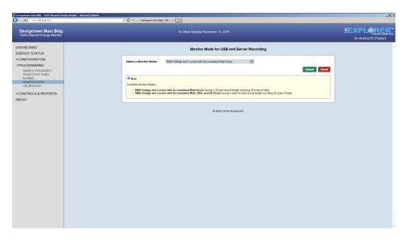
There are two fundamental monitor modes the first being the smallest record size recording only the basic information of voltage, current and watt hours occupying 32 bytes per record and thus allowing to store the maximum amount of records on the USB Flash drive. The extended mode records in addition reactive power and VA.
