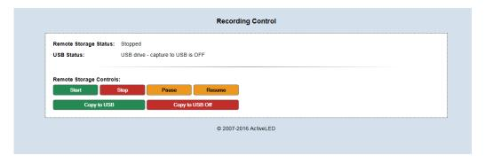
Start and Stop - Normally used to begin and end a sampling session recoding to the USB.
