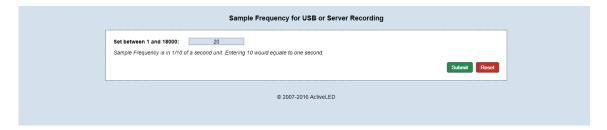
The sample frequency determines how often a sample is reported. At 18000, one sample is taken every 30 minutes. At 10, one sample is taken per second. At 1, ten samples are taken per second. The default value is 20, the equivalent to a 2 second sample rate.
